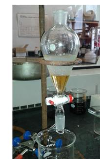
Extraction Set-Up Using brine and  $CH_2Cl_2$
