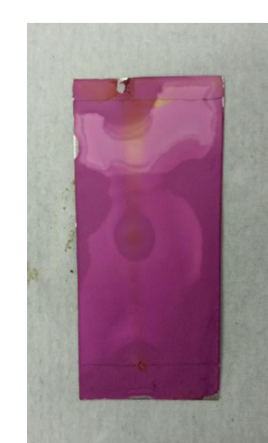
Figure 5. TLC of reaction progress from alcohol to ether
