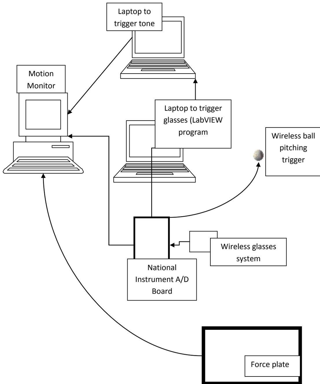
**Figure 3.1.** Instrumentation set up
